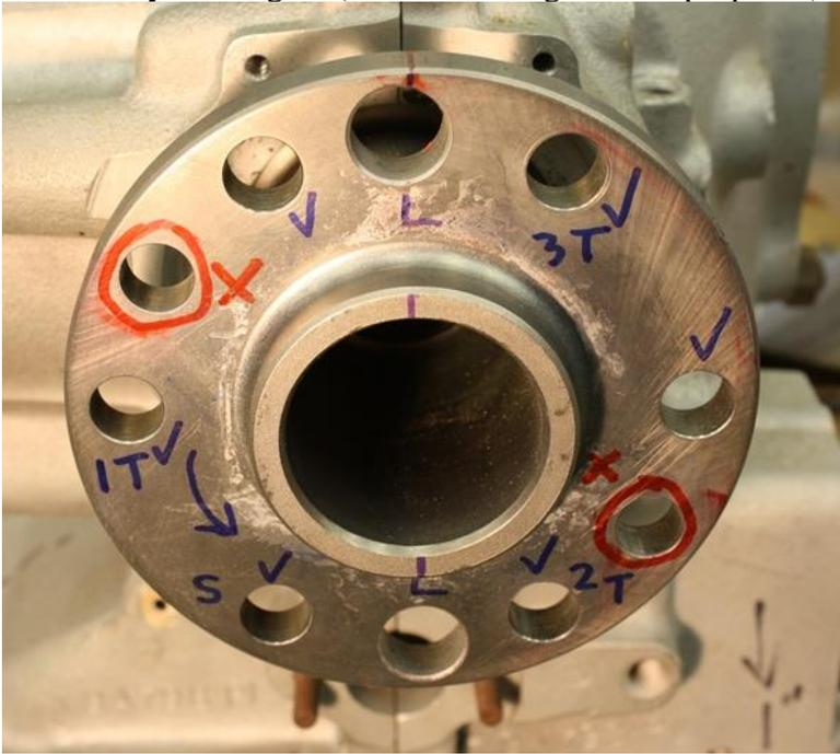
Magnet/ bolt placement on crank flange with crank at TDC 1
