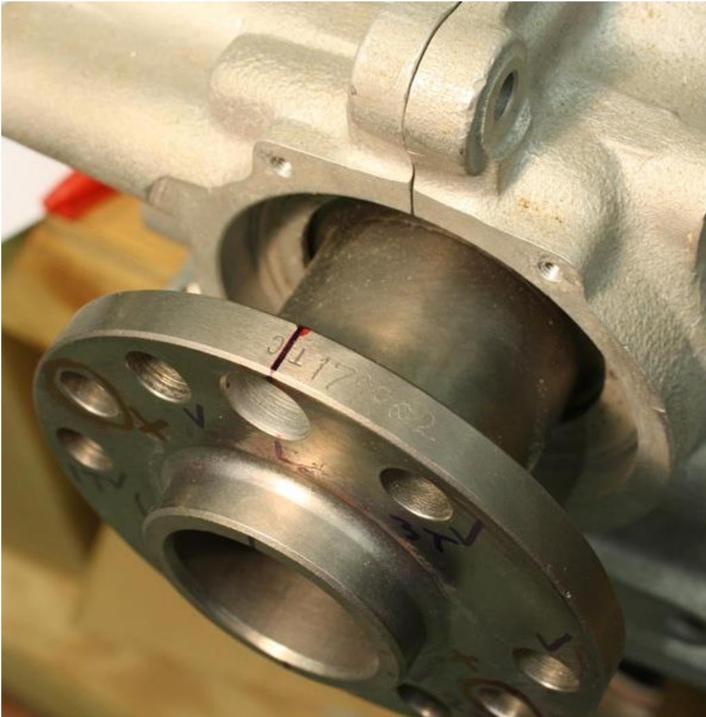
Put a white mark on the edge of the prop flange at the T/C mark
