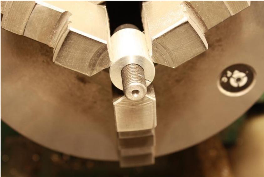
Using the drilling sleeve to clamp prop bolt in lathe chuck
