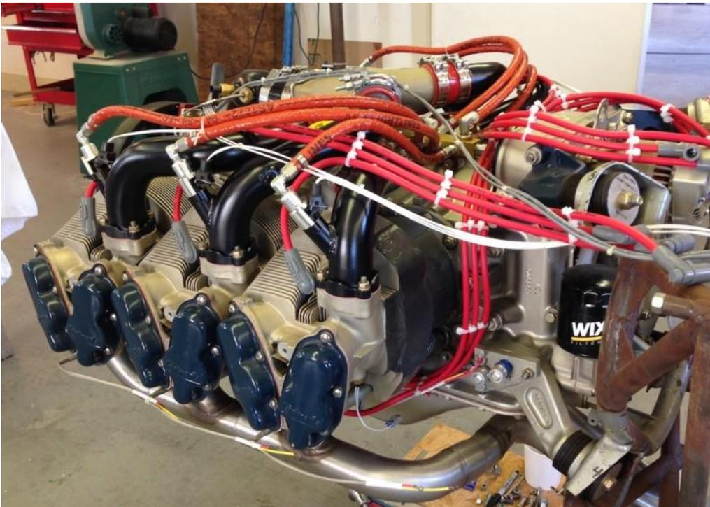
Locate the weld-on injector bosses near the ports on each intake runner in turn so that you have clearance to the cowling and room for the fuel fittings and injector electrical connectors. Using a Sharpie marker through the center of the boss, mark the central point on the runner. Pilot drill the mark with a 1/8 drill and then enlarge the hole with a step drill to 3/8. Use a 13/32 twist drill to oval the hole to match the injector boss footprint by
