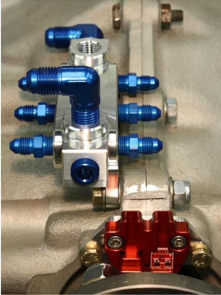
Screw in the supplied fittings as desired using a SMALL amount of Teflon pipe sealant compound Just enough to fill the threads of the fittings). NEVER use silicone (RTV) for sealing fittings! Tighten the fittings until snug and orientated as desired. Fuel should enter one end of the block through the AN6 fitting and head to the regulator from the AN6 fitting on the other end. There is provision for a fuel pressure takeoff as well.
