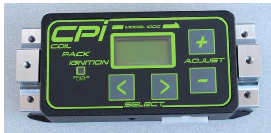
Blocks installed on CPI
