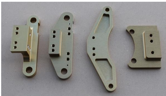
Left to right, Lycoming 4 and 6 cylinder Hall sensor mounts, Rotax 912, Jabiru 2200/3300
