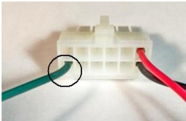
The Tach output wire(circled in photo) goes to the dash tachometer signal input.
