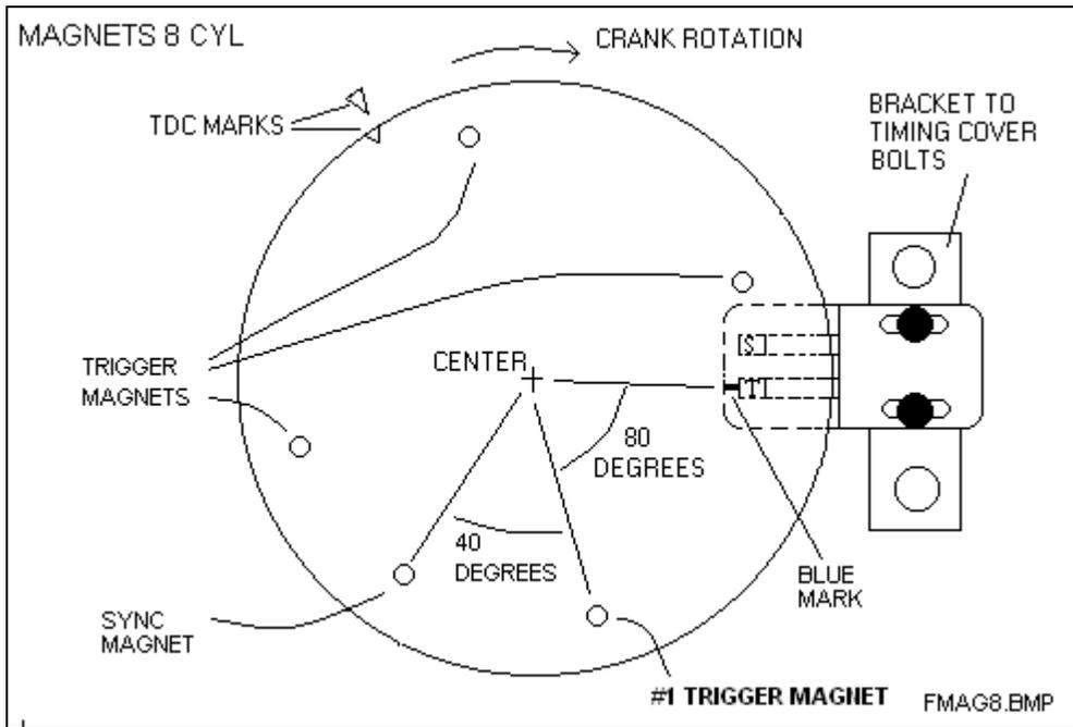
Schematic top view of hall sensor, pulley and bracket.
