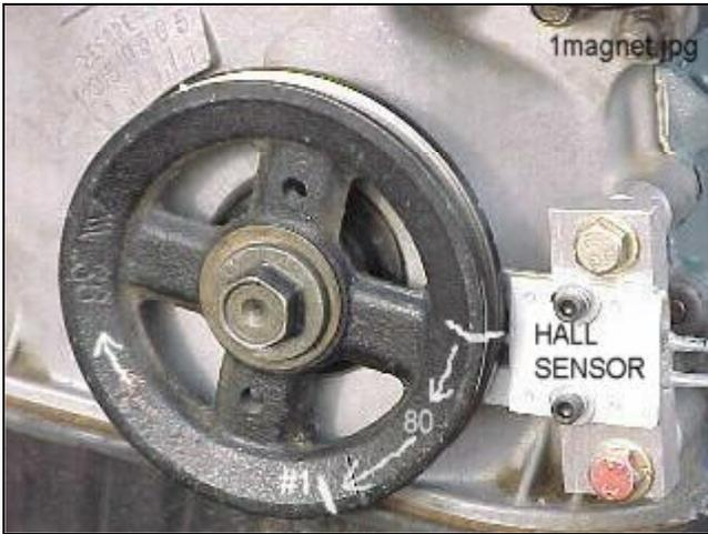
In this example, the engine rotates clockwise as shown by the arrow marked on the pulley. If this engine happened to rotate counter-clockwise, like a front-drive Honda, then the #1 magnet mark would be at roughly the one-o'clock position on this particular engine shown.
