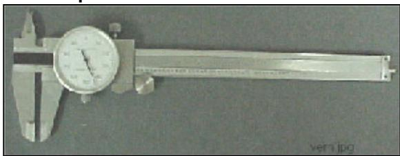
Use this end to check hole depth when drilling holes for magnets
