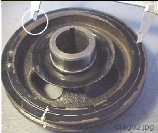
Scribe the last point with calipers and center punch this location for drilling.
