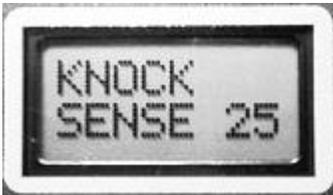
This value is used to adjust the sensitivity of the knock sensor circuit. This is adjustable between 1 and 32, with 1 being least sensitive.
