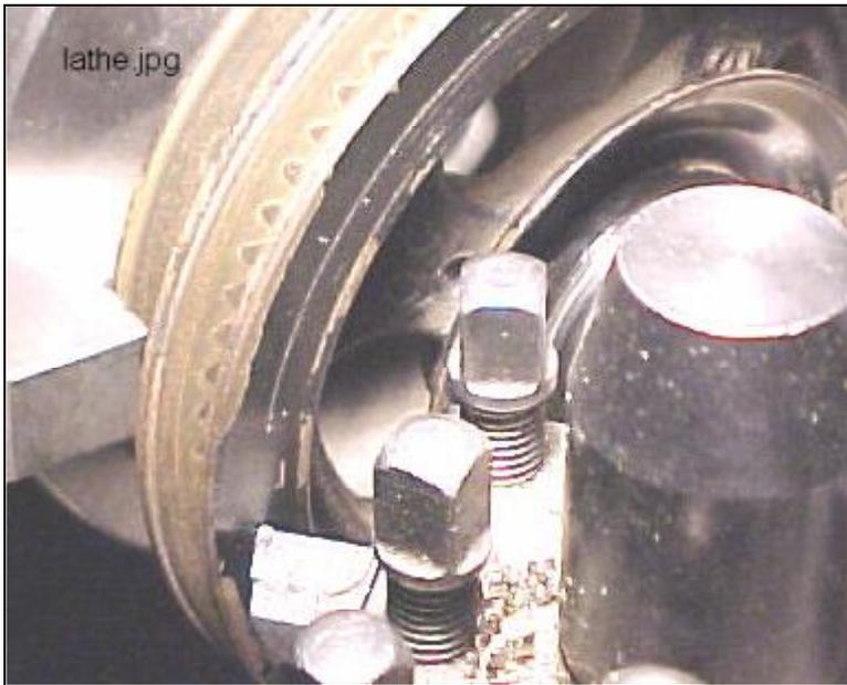
Pulley in the lathe. We recommend that you don't run the lathe motor, just rotate the chuck by hand slowly, with only light pressure on the cutting tool.
