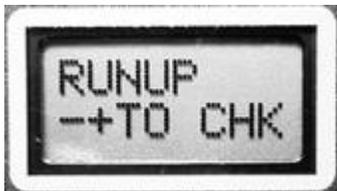
Intended for aircraft with twin plug engines to test operation of CPi coil pack(s).
