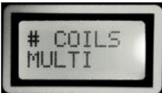
Multi or Single. Multi is used with coil pack or coil-on-plug. Single setting is for engines with a distributor where the CPi unit is triggering just one ignition coil.
