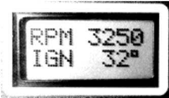
There are 38 RPM Ignition windows, above is one of them, 3250 rpm, where ignition is programmed at 32 degrees BTDC. These are where the main ignition programming of the system is done. For example, if you want timing at 20 degrees BTDC at 2500 RPM go to RPM IGN 2500 and enter 20. Etc.
