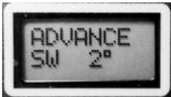
This option allows a dash mounted switch to activate the additional ignition advance timing programmed into this screen. The switch connections are one side to +12 volts, and the other side of the switch into pin12 via a blue wire.
