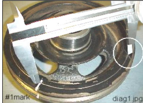
Scribe another arc at the top. This point is 180 degrees from the #1 Trigger magnet mark on the pulley. This point can be center punched for drilling.
