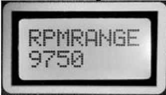
Allows selection of RPM range resolution. 4500, 9750 or 15,000 rpm can be selected. If say 9750 is used, you can still rev higher, but the highest programmable range would be at 9750, so this timing value will be used beyond 9750, up to as high as you rev the engine. 15,000 should be selected if RPM IGN values need different programming above 9750 rpm.
