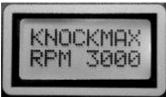
This disables the knock sensor above the RPM setting. This will prevent knock retard from occurring at higher RPM's, typically above torque peak rpm on most engines, since at very high RPM's, there may be a lot of engine noise picked up by the knock sensor. Leave at a really high setting if you don't want knock disabled.
