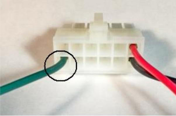
The Tach output wire(circled in photo) goes to the dash tachometer signal input.
