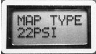
22PSI will be the automotive setting. 74" HG will be the aircraft setting. There are a variety of other settings for sensors which can be externally connected.
