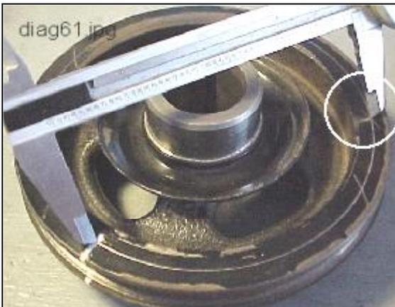
Scribe an arc with calipers and center punch this location for drilling.
