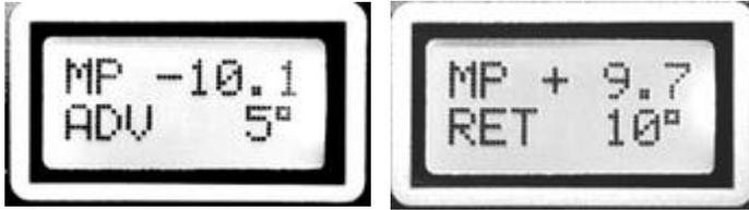
These 64 settings allow programming of ignition retard or advance with reference to load on the engine. Load information is from the MAP(MP) sensor. On systems not using a MAP sensor, the throttle position sensor is used for load information. RET refers to retard, and ADV refers to advance.
