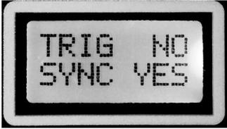
Top line is used for checking trigger magnets.
