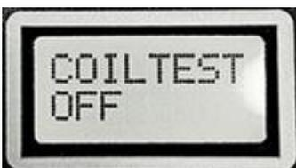
This screen turns on coil test by pressing +1, turns off with -1. Remove all spark plug wires and place them close to ground so the spark can jump.
