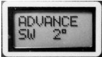
This option allows a dash mounted switch to activate the additional ignition advance timing programmed into this screen. The switch connections are one side to +12 volts, and the other side of the switch into pin12 via a blue wire.
