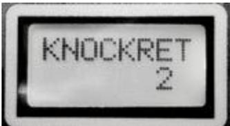
This value tells the CPi how much to retard the timing when a single knock event is sensed. A value of between 2 and 5 is recommended here.
