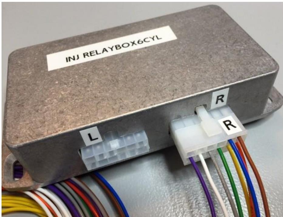
Figure 3. Injector relay box 6cyl. Note blue and brown wires from Mixture Knob Relay plug into pins 7 and 8, upper right corner of right connector.
