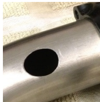
Make oval hole in induction tube
