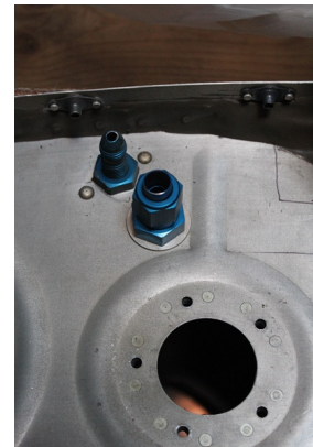
Return line using Earls Stat-o-seals
