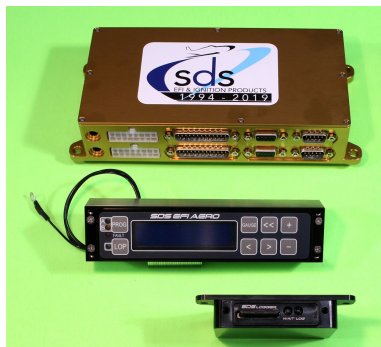
Dual EM-6 ECU with Design1 programmer and SDS card data logger shown
