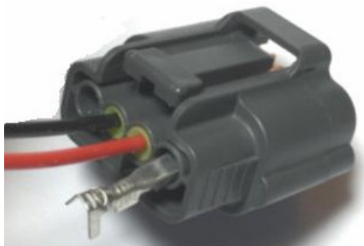
WITH CONNECTOR LATCH UP, AFTER CRIMPING YOUR WIRES INTO TERMINAL, INSERT TERMINAL INTO CONNECTOR WITH CRIMP FOLDS DOWNWARD.
