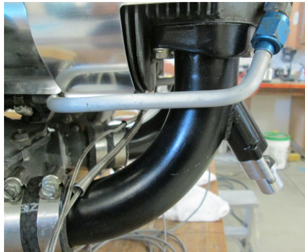
Injector boss welded in place ( Lycoming)
