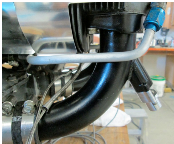
Injector boss welded in place ( Lycoming)
