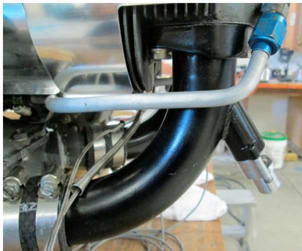
Injector boss welded in place (Lycoming)
