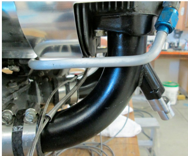
Injector boss welded in place (Lycoming)
