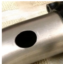
Make oval hole in induction tube
