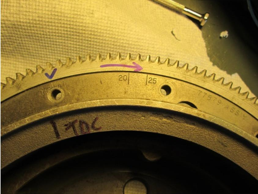
2. Now viewing the flywheel from the back side, counting the hole closest to the TC#1 mark as 1, use marker to mark all twelve 1/4 inch flywheel holes as shown below:
