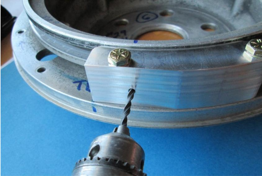
This hole is for the #1 trigger magnet
