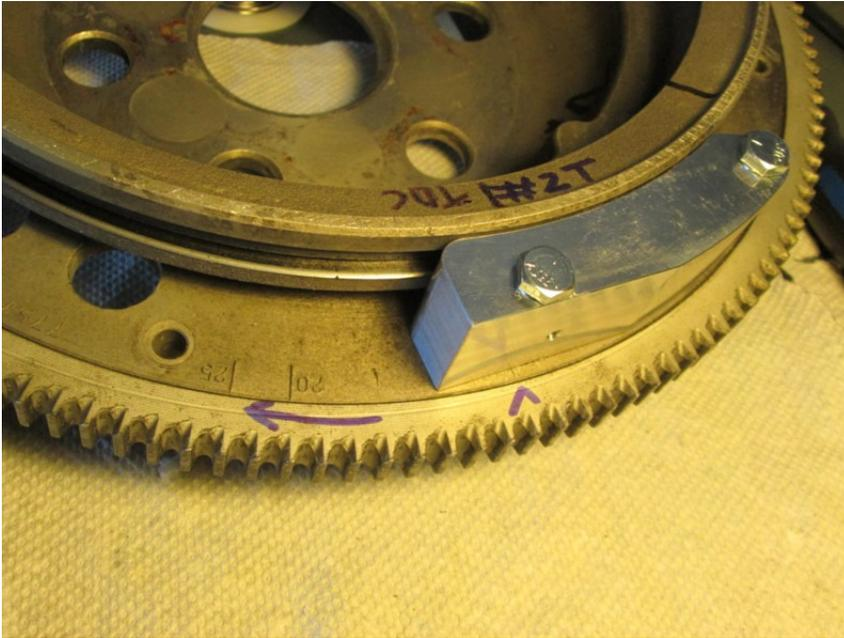
8. This is the #2 Trigger Magnet hole and should be 180 degrees across from the #1 Trigger Magnet hole. Mark this hole as “2T”. Drill through the flywheel.
