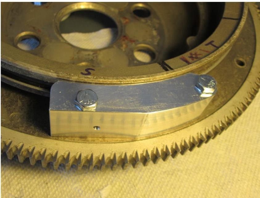
7. Now, move drilling block over so that drilling hole is close to the “TC #1” mark on rear of flywheel. The block should be over holes 12 and 1. See photo below.
