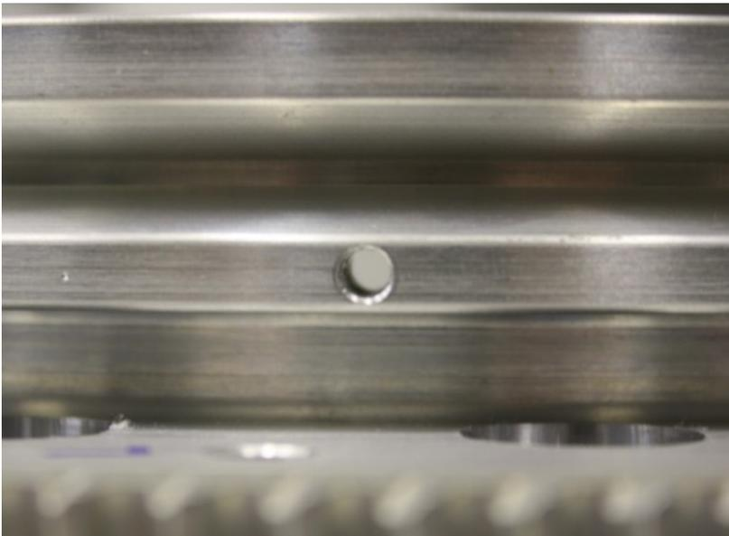
5. Use the supplied #29 drill to drill through the drilling block and flywheel as shown below. Lubricate the drill and remove frequently to clean out the chips. Mark the flywheel close to the hole as "1T" with marker.
