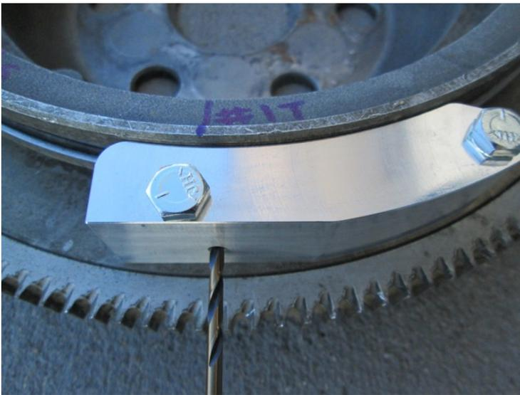
This hole is for the #1 trigger magnet
