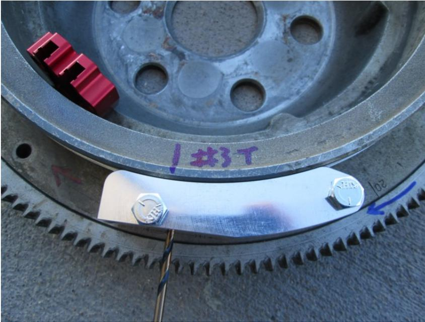
Remove the drilling block and insert the supplied 8-32 tap, lubricated with tap oil, into each drilled hole. CAREFULLY tap until the tip of the tap is flush with the ID of the flywheel, don't tap all the way through. Break the chips on every turn of the tap and clean the tap and hole of chips with compressed air frequently to prevent jamming and breaking the tap. Clean the holes out with acetone to remove all traces of oil.
