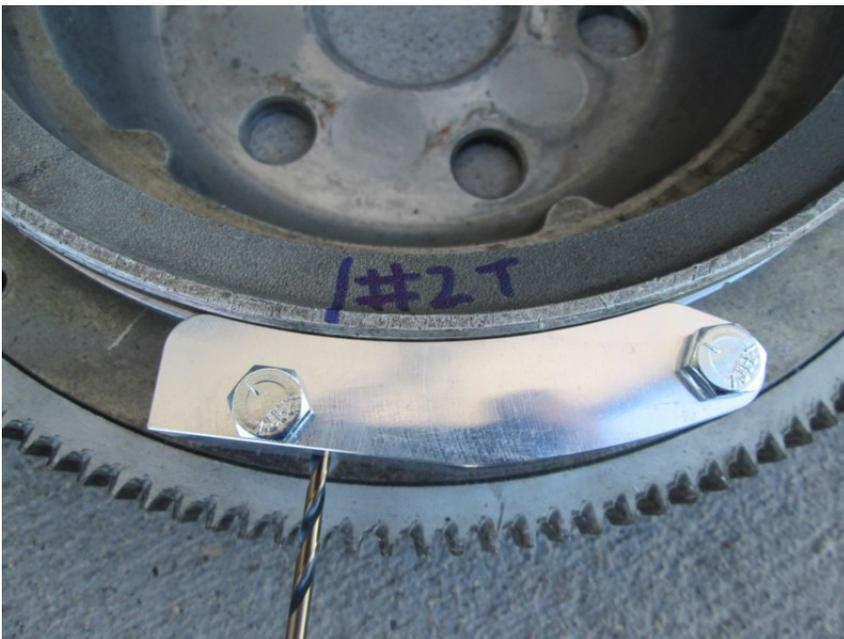
6. This is the #2 Trigger Magnet hole and should be 120 degrees across from the #1 Trigger Magnet hole. Mark this hole as “#2T”. Drill through the flywheel.
