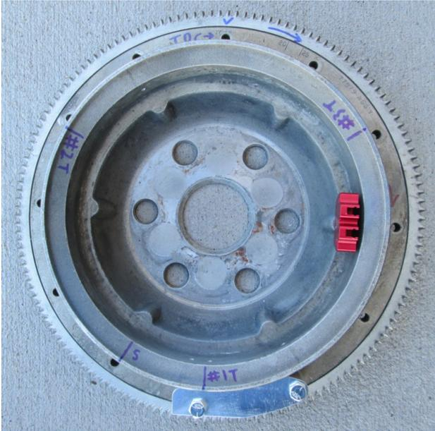
We recommend that you number each of the twelve 1/4 inch holes in the flywheel with marker as shown below starting at the TC#1 hole as 1.
