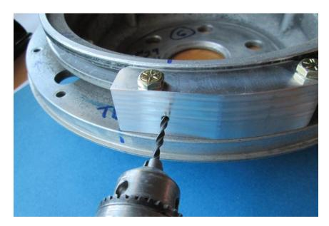
This hole is for the #1 trigger magnet
