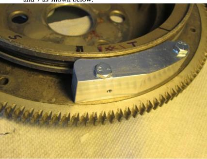
3. Use the supplied #29 drill to drill through the drilling block and flywheel as shown below. Mark the flywheel close to the hole as "1T" with marker.
