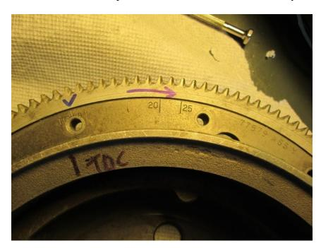
2. Now viewing the flywheel from the back side, counting the hole closest to the TC#1 mark as 1, count over 6 holes in the direction of crankshaft rotation (clockwise as viewed from the BACK of the flywheel). Line the round edge of the drilling block with this hole, slip the supplied bolts through the block and holes 6 and 7 as shown below.
