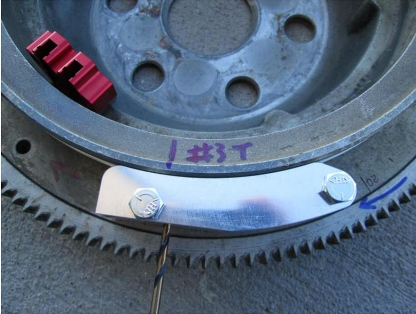
Remove the drilling block and insert the supplied 8-32 tap, lubricated with tap oil, into each drilled holes. Carefully tap all the way through the flywheel until the last flutes on the tap reach the outer edge of the flywheel edge. Clean the tap of chips with compressed air after each hole and clean the holes out with acetone.
