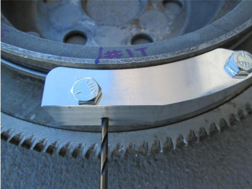
This hole is for the #1 trigger magnet
