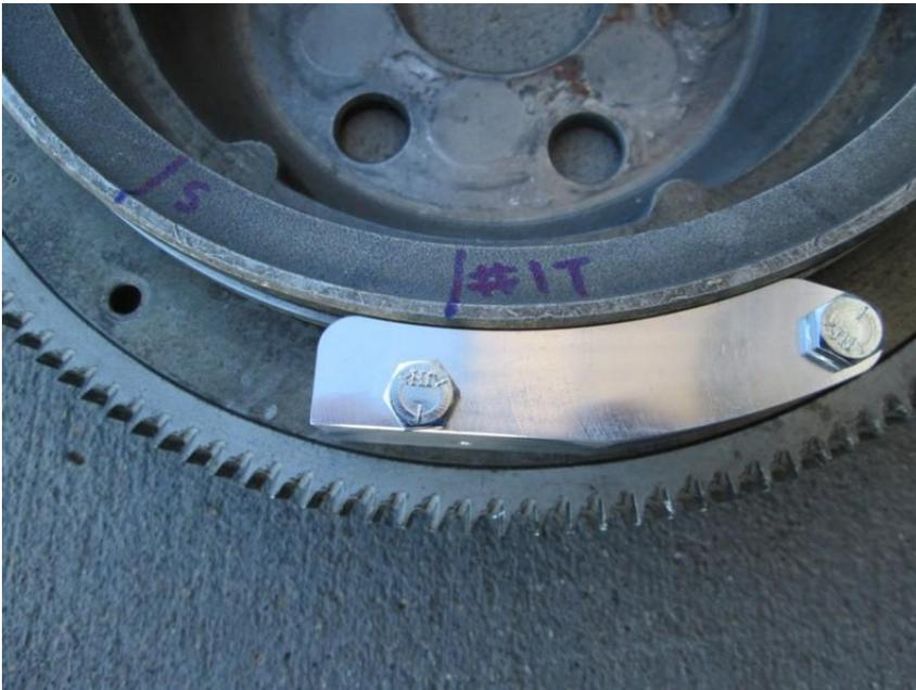
3. Use the supplied #29 drill to drill through the drilling block and flywheel as shown below. Mark the flywheel close to the hole as “#1T” with marker.
