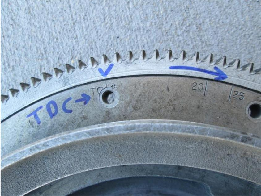
1. Now viewing the flywheel from the back side, counting the hole closest to the TC#1 mark as 1, count over 6 holes in the direction of crankshaft rotation (clockwise as viewed from the BACK of the flywheel). Line the round edge of the drilling block with this hole, slip the supplied bolts through the block and holes 6 and 7 as shown below.
