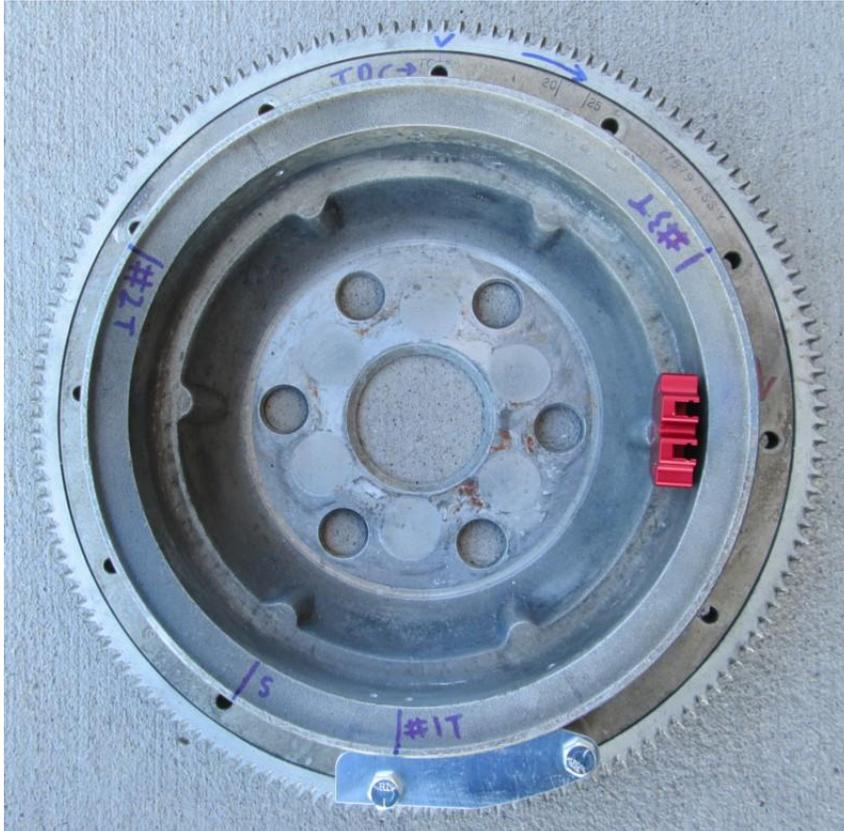
1. Locate the TDC mark on the Back side of the flywheel, stamped TC#1 as shown below.
