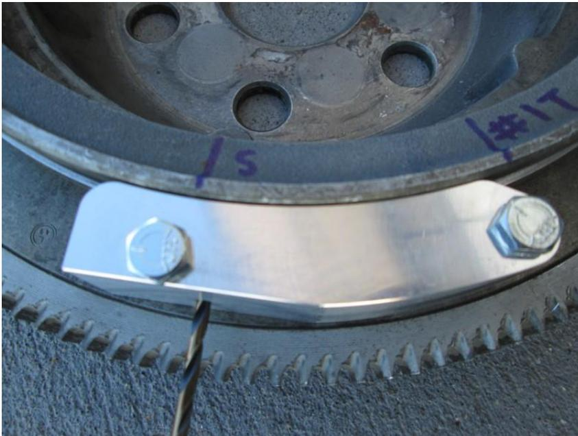
5. Now, move drilling block over so that bolts go through holes 10 and 11. Mark this hole as #2T.
